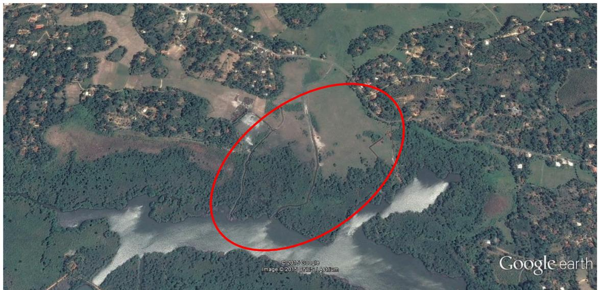
Figure 2. Enlarged area (N 06 00 859; E 080 20 628) to show the two water canals that can be cleared to increase the flow.
